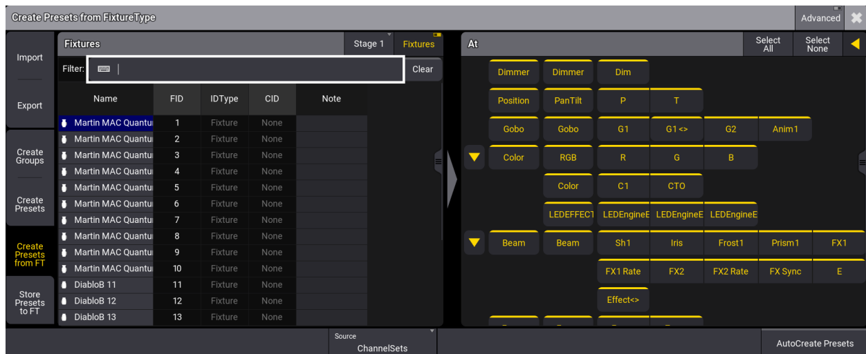
Create Presets from FT menu with Fixtures enabled and expanded At Filter area
